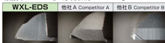
切削長さ4.2m時の摩耗状況 After Milling 4.2m
