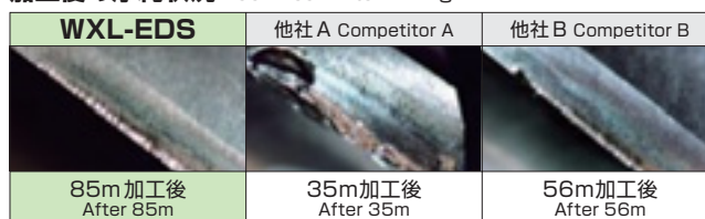
加工後の摩耗状況 Tool Wear After Milling
